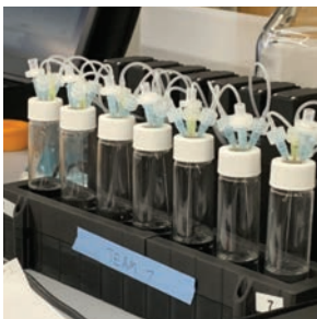
Participants in Genomics use a chemostat to stimulate evolution of antibiotic resistance, then analyze the mutated genome.
